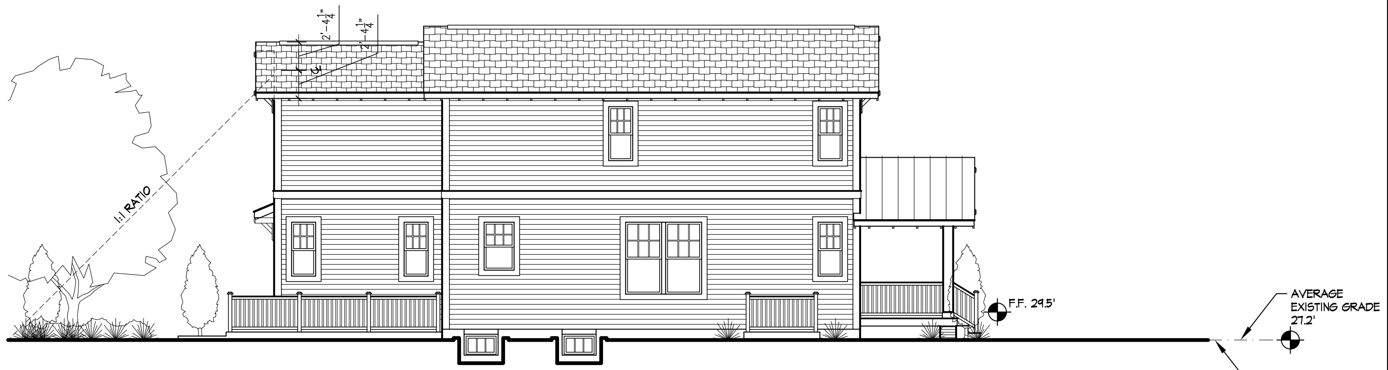
2 PROPOSED NORTH ELEVATION A7 SCALE: 1/8" = 1'-0"
